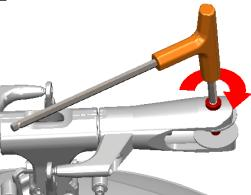
Check main hub screws(M4x24 and 2 M3x12) Ensure they are tight.
