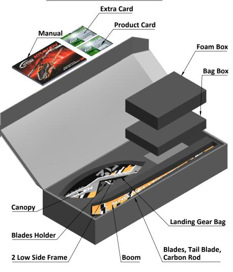
The assembly process is described in the following chapters. Each chapter provides you with the box, bag and/or foam numbers you will need for that chapter. The information is printed in a black box in the upper corner of the page.
