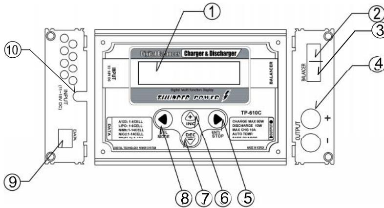
1: LCD screen 2: Upgrade connector 3: BL-2 (balance tap) connector 4: Charge Output 5: Enter/Stop button 6: INC button
