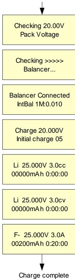
Lipoly charging sequence is shown below. Each step is specially designed for the safe lipoly charge algorithm.
