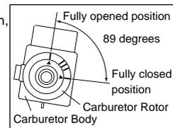
When the triangle mark on the carburetor rotor meets the far right mark, the throttle is fully closed. When the triangle mark meets the top mark, the throttle is fully open. The range is 89 degrees. You may use the other three marks as the reference marking of throttle opening to your preference when hovering.
