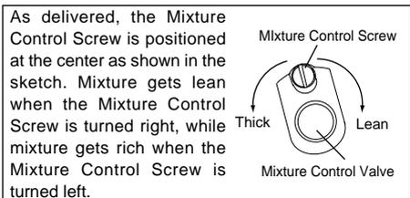
As delivered, the Mixture Control Screw is positioned at the center as shown in the sketch. Mixture gets lean when the Mixture Control Screw is turned right, while mixture gets rich when the Mixture Control Screw is turned left.
