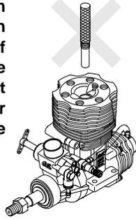
It is recommended to use Crankshaft Clamp 7091 (Code No.71530500) available as an optional tool. It is made of durable engineering plastic and locks the crankshaft without risk of damage to any part of the engine.
