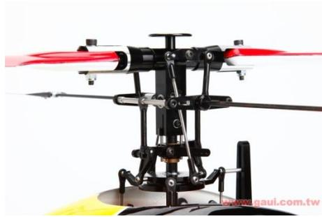
When the throttle stick is advanced power increases along with an increase or decrease in main blade pitch
