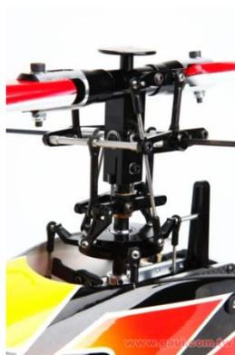
Fore and Aft Cyclic Moves the swash plate from front to back and back to front
