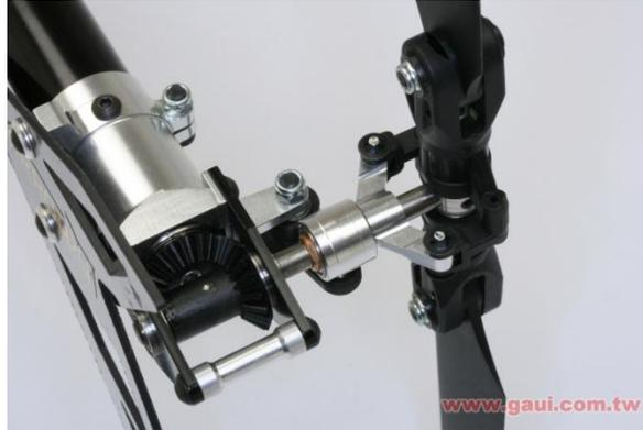
Tail blade pitch controls direction of nose rotation
